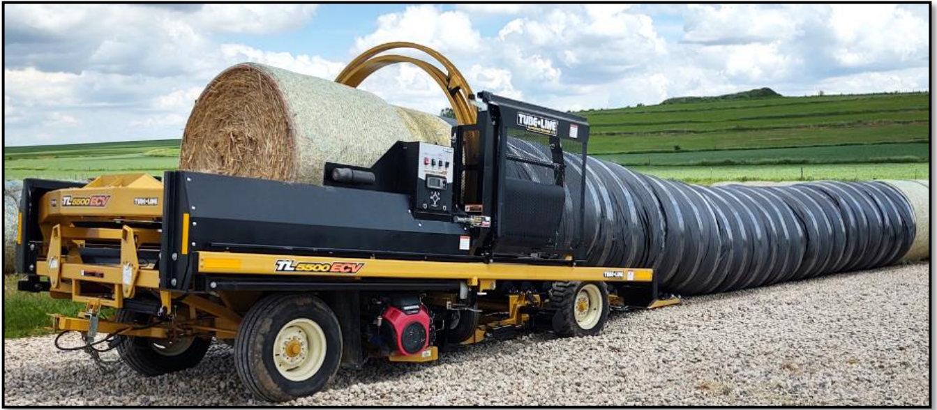
Figure 3. Dry alfalfa bales wrapped in breathable film using the modified bale wrapper. Note spiral wrap of tape at the training edge seam to seal the film.
